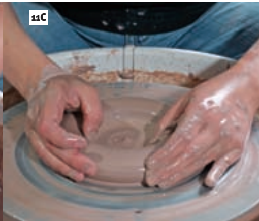
Opening the clay further with thumbs.
