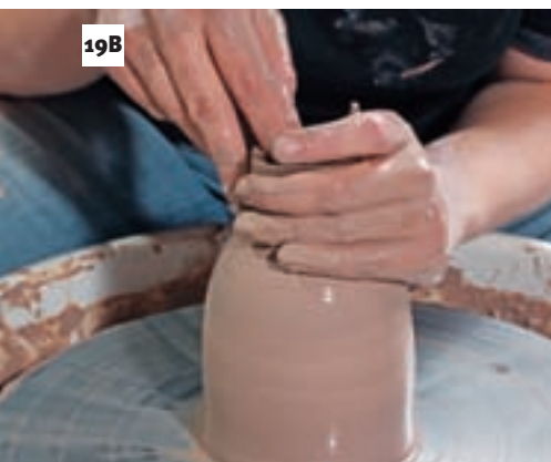
As collaring progresses the neck gets gradually more narrow.
