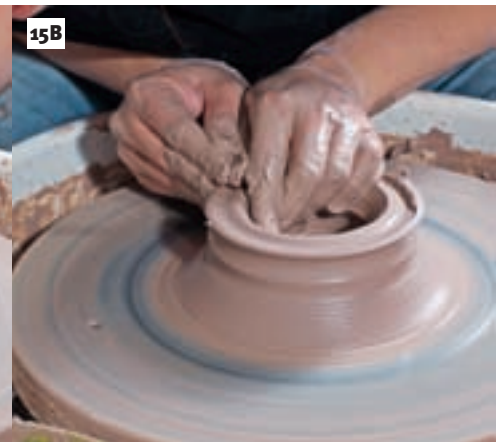
Pulling the walls up. You can see the bulk of the clay as a ring being pulled to the top.
