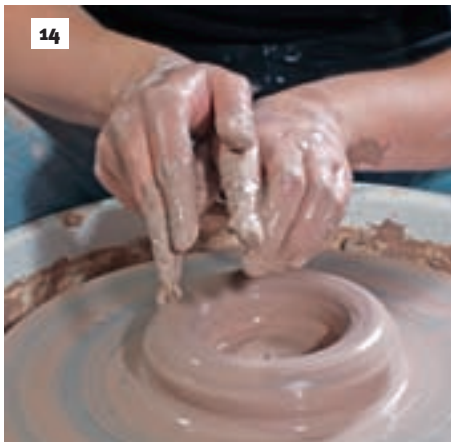
This is a good hand position when learning to pull up the walls of a pot. Keeping your hands together will minimize wobbles.
