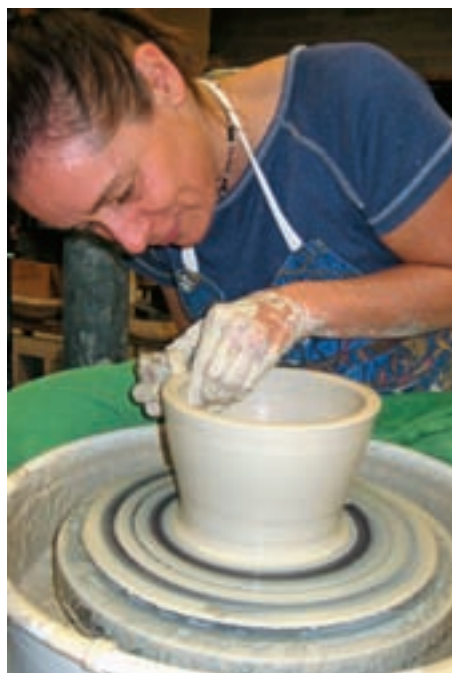
Pulling up the walls of a vessel.
