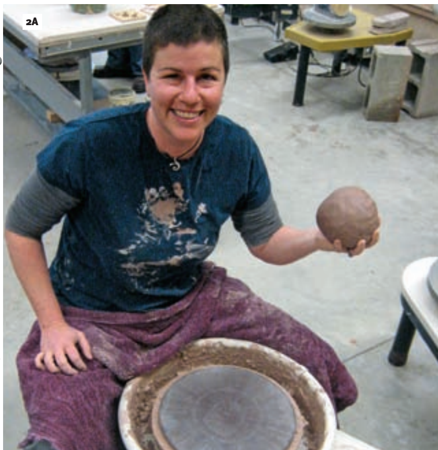
Once your clay is prepared, slap the ball of prepared clay onto the wheelhead as near the centre as you can.
