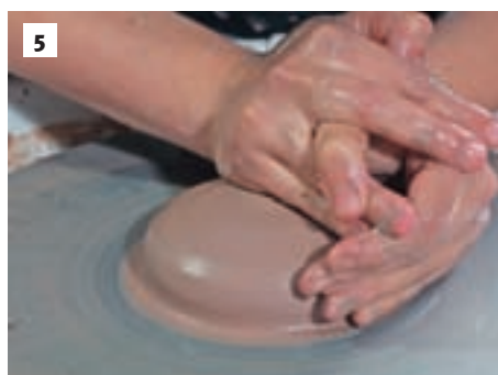
With wet hands, begin by pushing down on the top of the clay. This begins the centring process and helps further attach the clay to the wheel.
