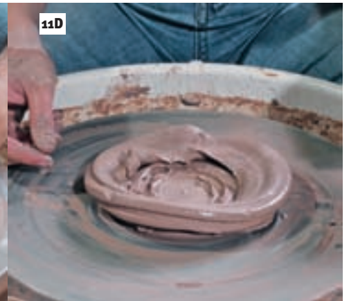
If you pull outwards too far at this stage, the top ring of clay will come off the base. Time to start over.
