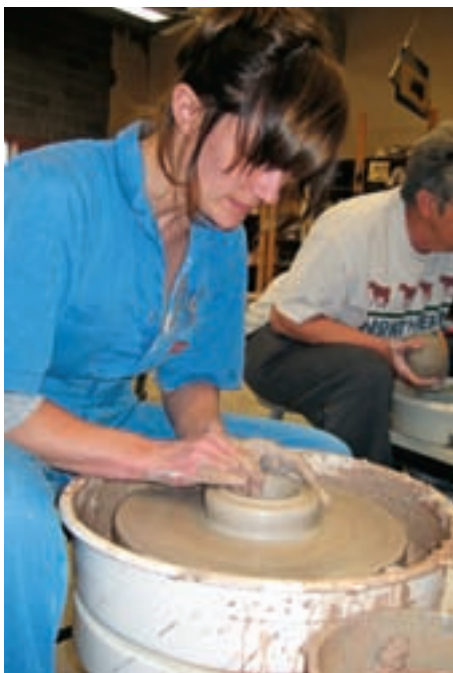
Opening up the clay to create a base for a pot.
