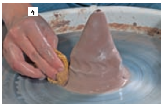
Use your sponge to completely seal edge of clay to wheel before adding water.
