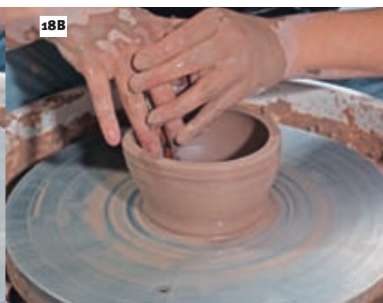
Beginning to shape a cylinder into a bowl using a rib. One of the curved sides of the rib is held against the inside wall.
