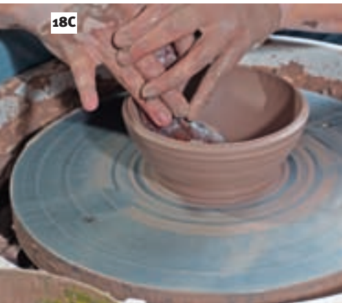
Continuing to shape a cylinder into a bowl using a rib.
