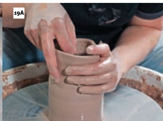
Collaring a cylinder to make the form narrower.
